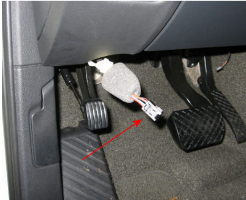
Figure 2. The four pin connector is located under the left lower dash. It falls down when the left lower close out panel is removed.
